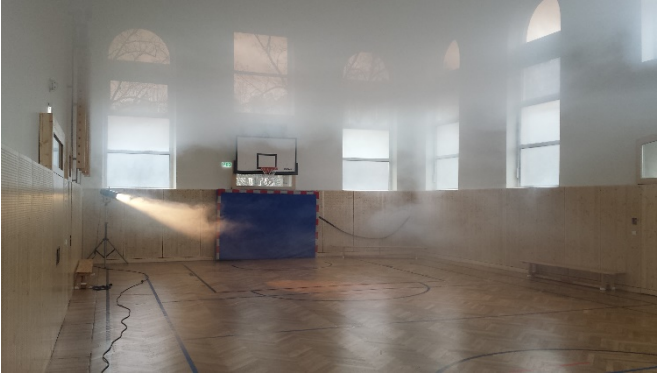
Smoke test 1: Without Climotion, air stratification occurs above the occupied zone.
