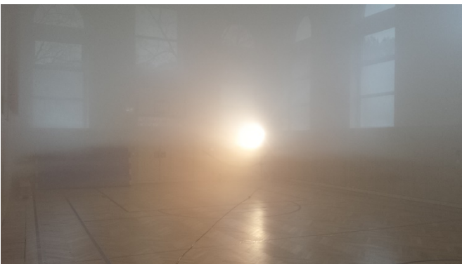
Smoke test 2: With Climotion, the system distributes the air evenly throughout the gym.
