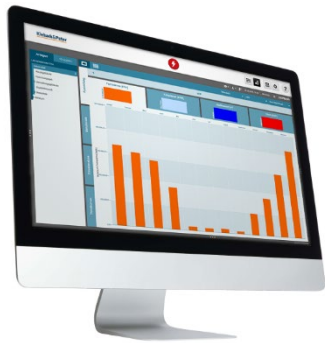
Energy and system data displayed in the Qanteon building and energy management system from Kieback&Peter. Starting in 2025, non-residential building automation and control systems for heating and air conditioning systems with a rated output of 290 kW or higher must do the following: meet benchmarks regarding the building's energy performance, detect efficiency losses in building services, and inform the building manager about possible improvements in energy performance.
